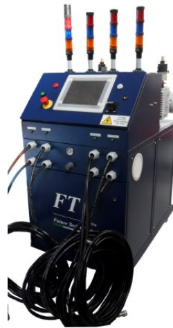
iAmiata for pressure stress test
