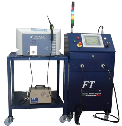
iAmiata connected to leak detector
