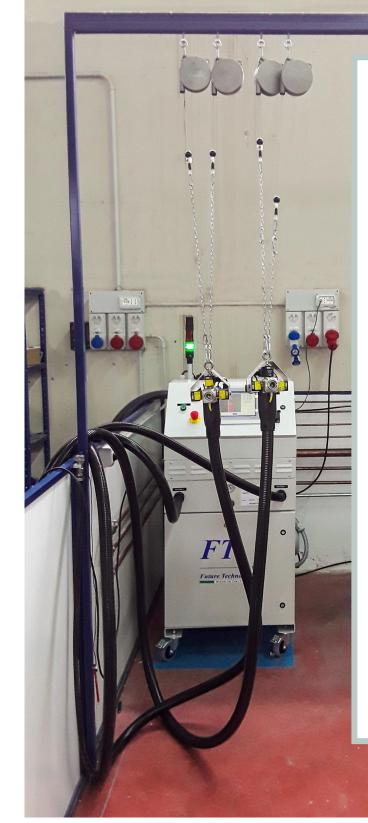
**The injector** is the connection device between the Refrigerant charging machine and the cooler refrigerant circuit.
